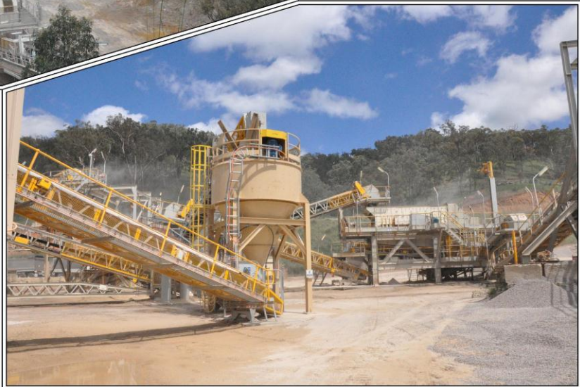
Plate 1.4: Section of the Processing Plant - Quaternary crusher is located in the left foreground (Ref: E652S_041)
